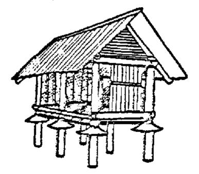
Fig, 53 Improved crib built from imported materials, Swaziland
