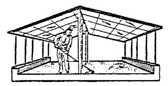
Fig. 22 Plastic-covered, walk through solar coffee dryer, Columbia
