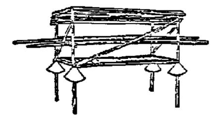
Fig. 17 Solar "chimney" fryer with pre-heater
