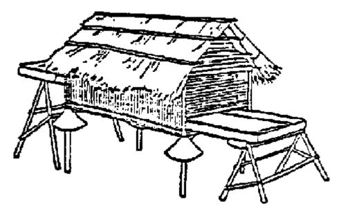
Fig 19 Walk-through, plastic-covered, solar coffee fryer, Columbia
